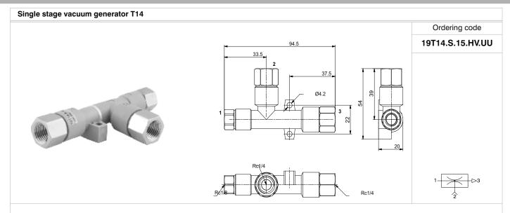
Single-stage generators, robust and reliable, with compact dimensions and suitable for applications which need the required degree of vacuum to be reached quickly with limited air flows. Operating on the Venturi principle, they have the vacuum connection, orthogonal to the axis of supply and outlet. They can be connected directly to the suction cups and/or suction cup holder and applied in any position.
