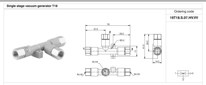
Single-stage generators, robust and reliable, with compact dimensions and suitable for applications which need the required degree of vacuum to be reached quickly with limited air flows. Operating on the Venturi principle, they have the vacuum connection, orthogonal to the axis of supply and outlet. They can be connected directly to the suction cups and/or suction cup holder and applied in any position.
